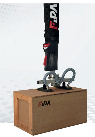
FIPALIFTpro with its unique control handle design, allows for powerful lifting of loads up to 75kg. The intuitive, ergonomic, easy to use single handed controls create a versatile, user friendly and powerful solution. Lift, lower and balance the load all with one hand.
