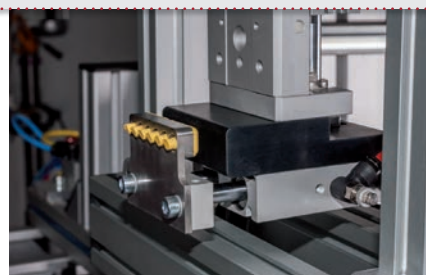
Combination of dual-piston cylinder and guide block
